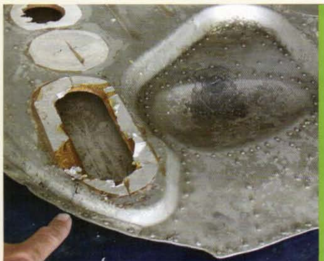
Crack in inner gear door....also intergranular corrosion has broken through. See hole in blister at center of door.
